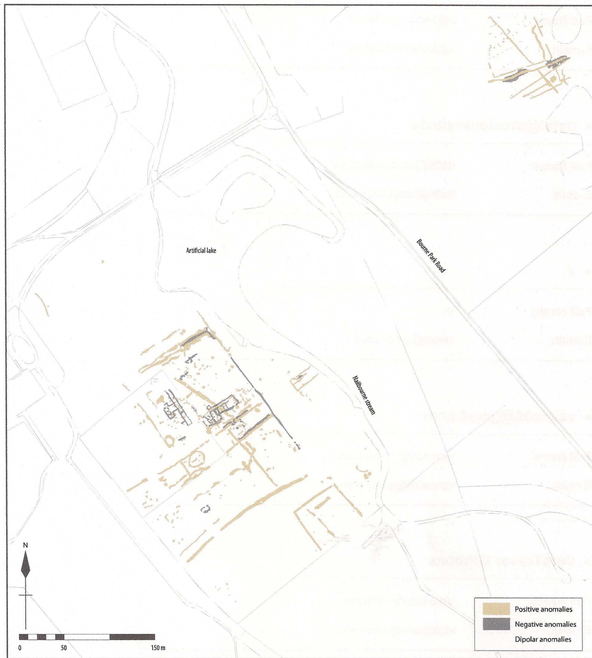
Fig. 13. Digitised anomalies detected in the gradiometer survey and Ordnance Survey topographical data.
