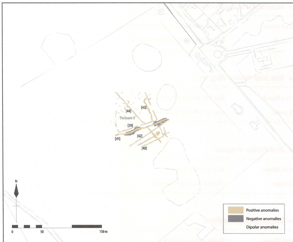
Fig. 16. Digitised anomalies detected in the gradiometer survey of Field 2 and Ordnance Survey topographical data.
