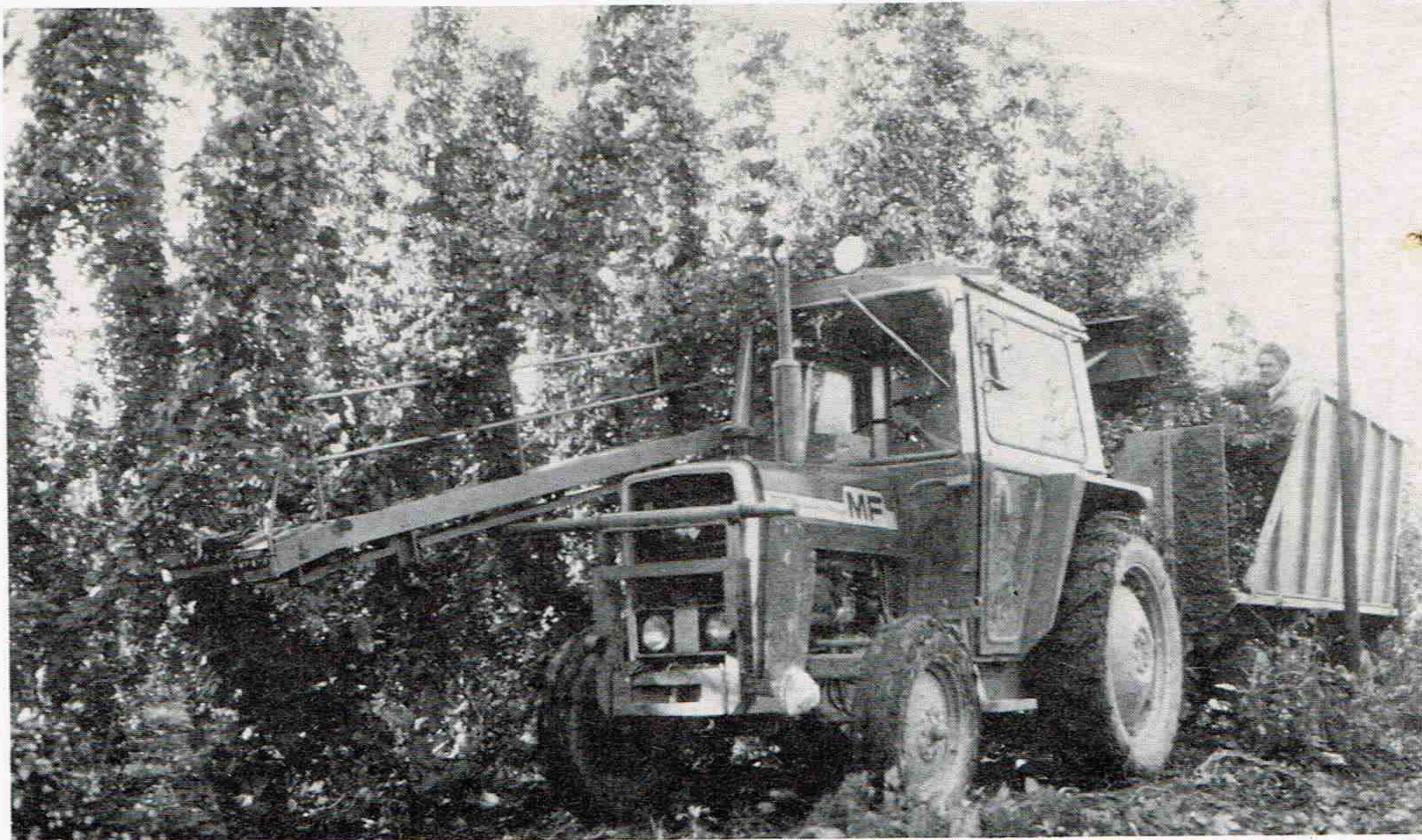
On a large brewery-owned hop farm in Hereford picking goes on 24 hours a day with a new machine (above) which clips the bines from the wires while people in the cart tug the bines from the wires. (Below) the higher the alpha acid content of a hop the more beer that it can flavour; a technician at the Hop Research Department of Wye College at Ashford in Kent does an alpha acid analysis
