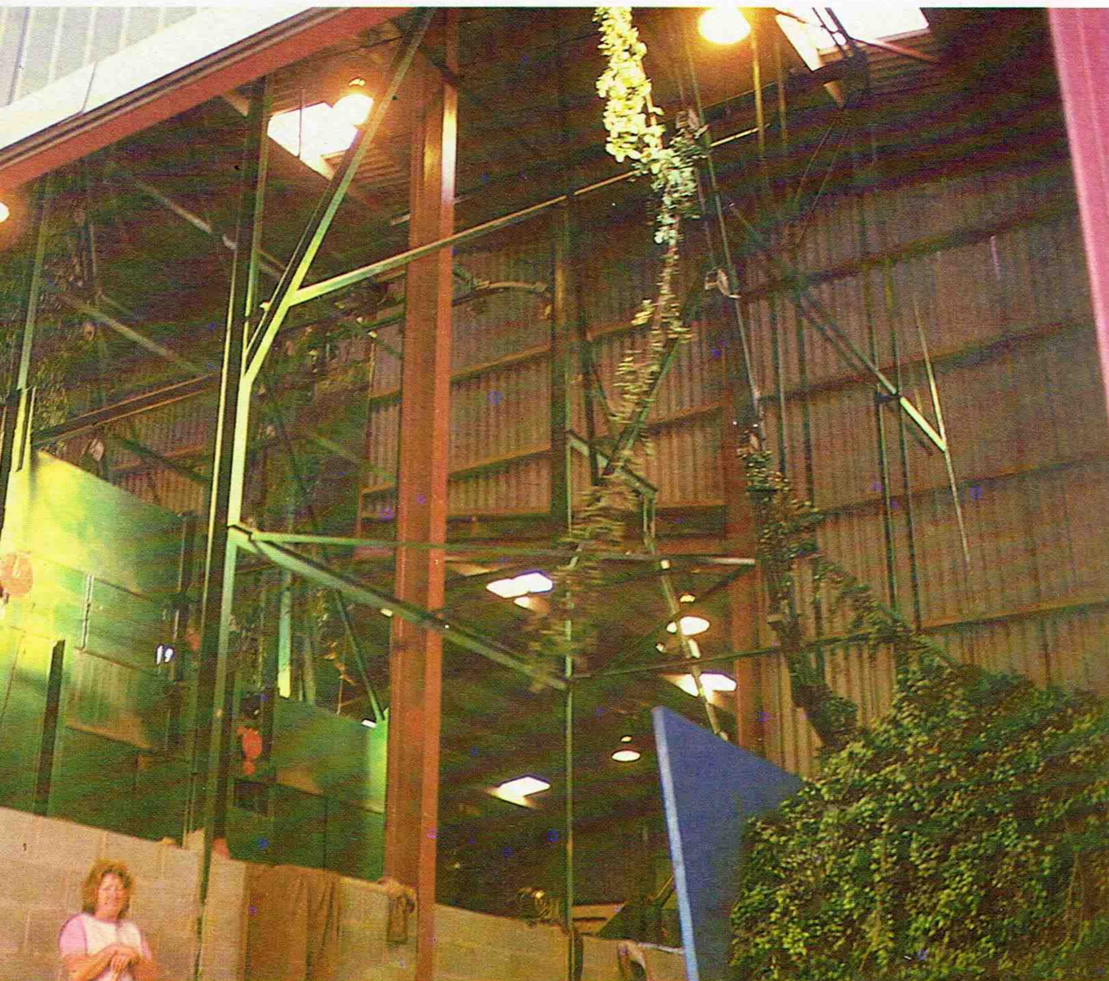
The bines are fed into a track conveyor at the brewery farm (above) while the waste from the plant is blown out to a storage area outside, from where it is taken to be used as compost for the next crop. The bines then pass between pairs of rotors which have tines that tease off the hop cones together with leaves and shoots (below left). A conveyor belt then carries the hop cones past cleaners (below right) who pick out any remaining waste
