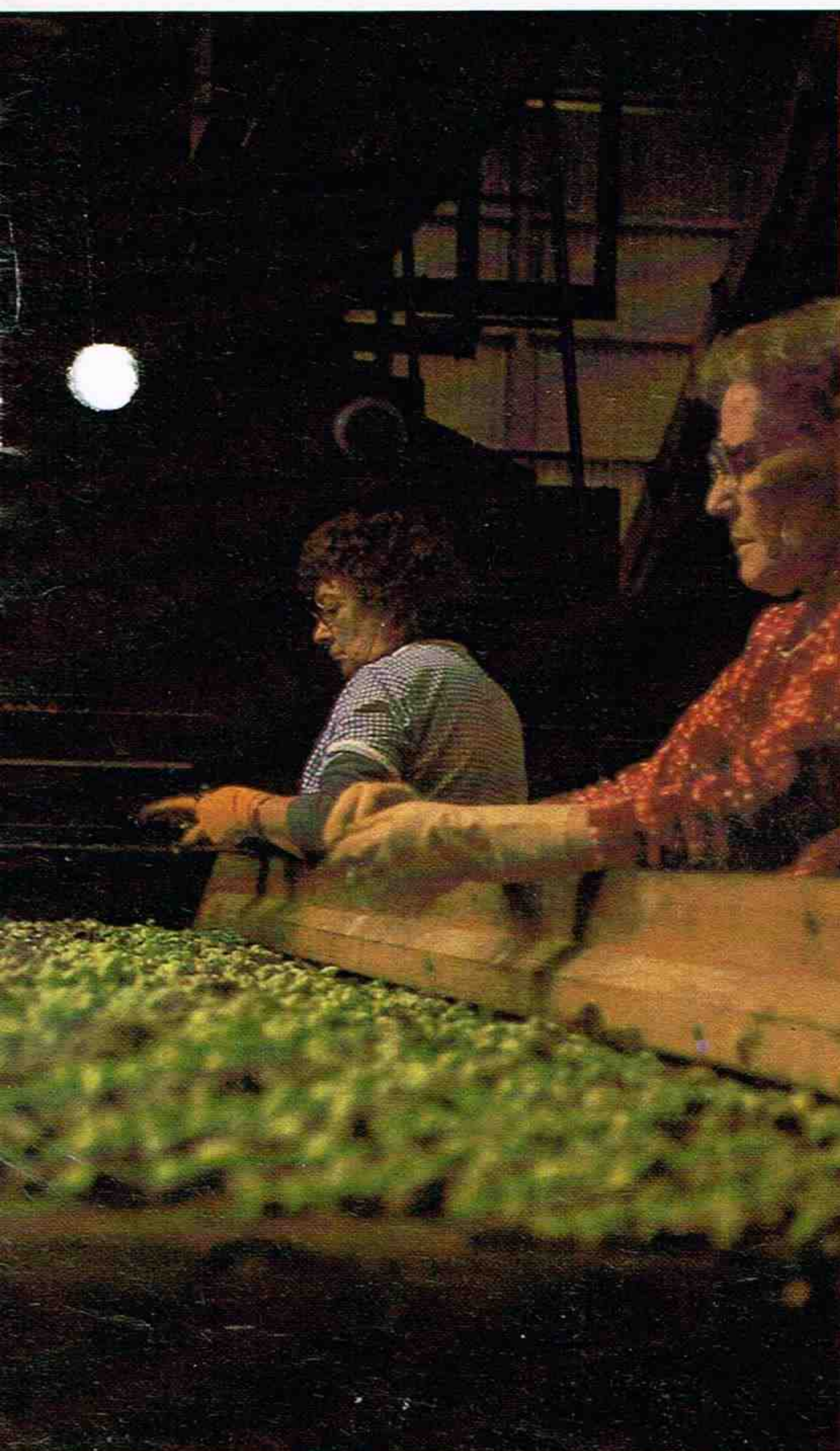
The cleaned hops move on by conveyor belt to a dryer (top right) which takes six hours to dry the hops at 60°C. The plant operates 24 hours a day
