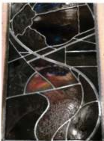
13. (right) The panel is loaded up and all the joints are soldered.
