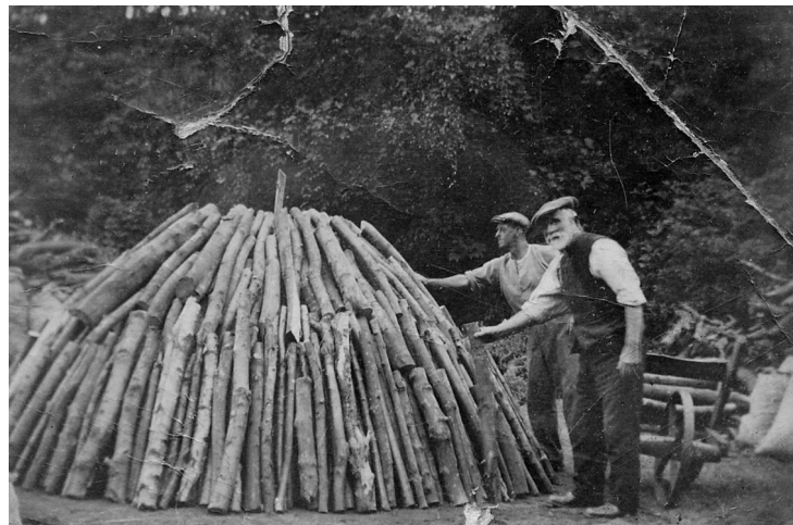
John Francis and son stacking the 'pit' ready for charcoal making (Alan Clayson)
